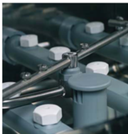
Superior cleaning action with 7 bayonet style wash arms with 42 fixed wash jets.
