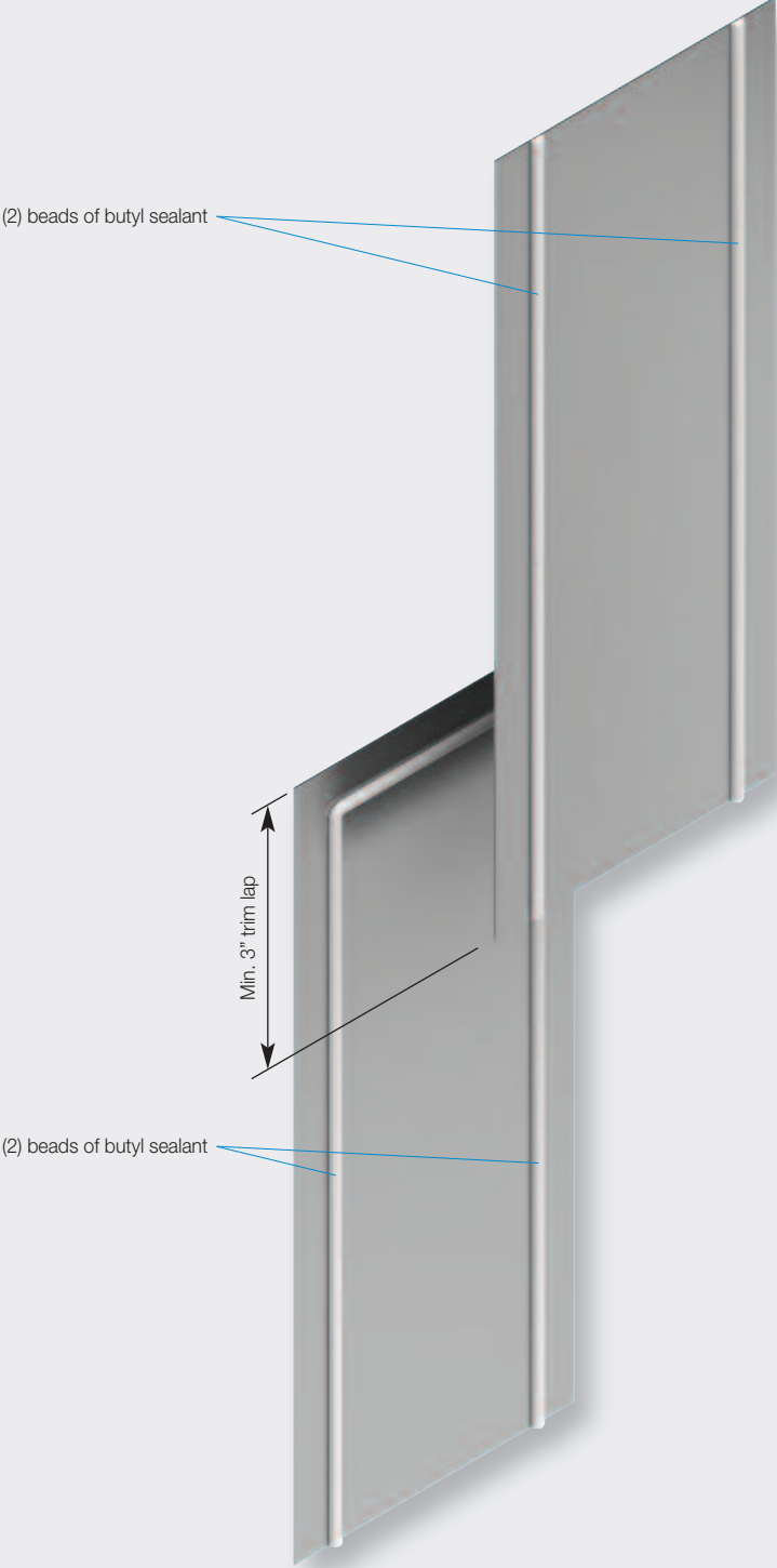
Mending Plate “Shingle” Lap Detail
