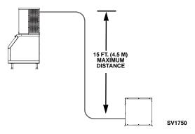
**15 ft. (4.5 m) Drop:** The maximum distance the CVD® Condensing Unit can be below the ice machine.
