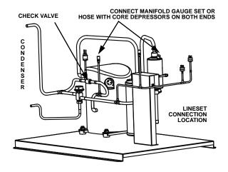
Pressure test the line sets and CVD® Condensing Unit with 150 psig of dry nitrogen. Add nitrogen at the line set shut-off valves located at the back of the ice machine head section or from the schrader valves located in the CVD® Condensing Unit. Complete the pressure test, verify no leaks are present and remove the nitrogen from the system before connecting the vacuum pump.
