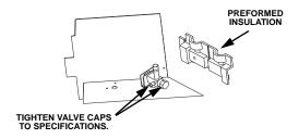
A. Verify valve and schrader caps are tightened to specifications (see step 6).
