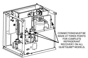
Refrigerant Recovery Connections Ice Machine Head
