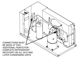
Refrigerant Recovery Connections CVD Condensing Unit
