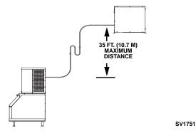
**35 ft. (10.7 m) Rise:** The maximum distance the CVD® Condensing Unit can be above the ice machine.
