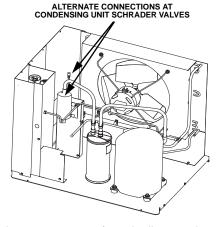
Isolate the vacuum pump from the line set shut-off valves and/or condensing unit access ports prior to proceeding.
