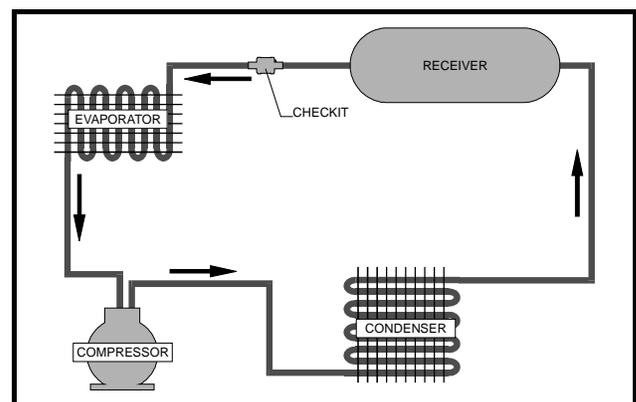
**Figure 12** - Typical Checkit Sensor Location
