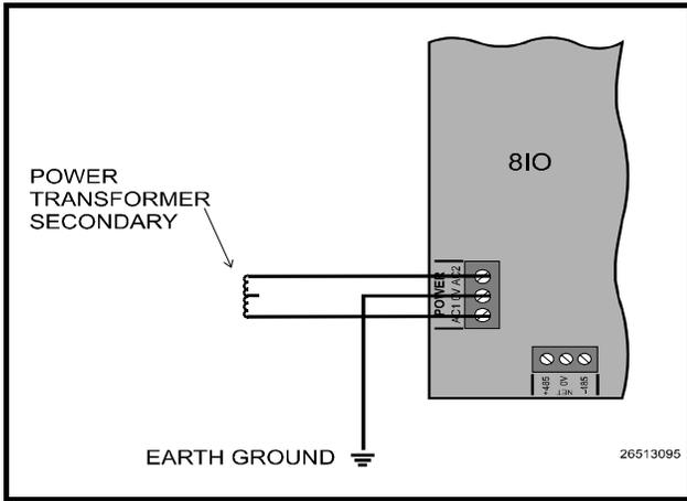
*Figure 39-Single 8IO Board Wired to One Transformer*
