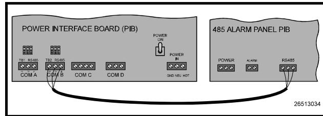
**Figure 3 - COM B Wiring - REFLECS to 485 Alarm Panel**
