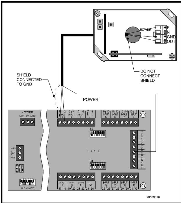
Figure 20 - Relative Humidity Sensor Wiring
