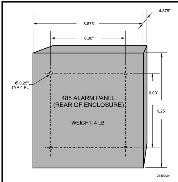
**Figure 2 - 485 Alarm Panel Mounting Dimensions**
