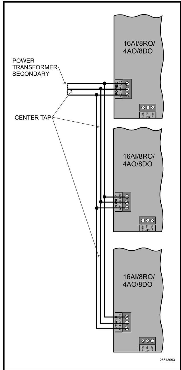
Figure 38 - Wiring for Three 16AIs, 8ROs, 4AOs, or 8DOs or Any Combination of
