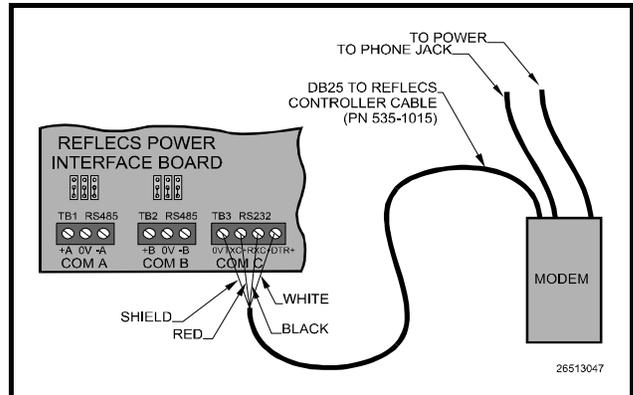
Figure 10 - COM C Network Connection
