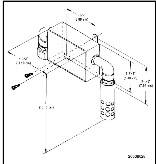
Figure 21 - Outdoor RH Sensor Mounting Dimensions
