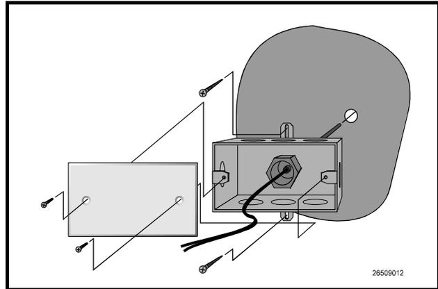
Figure 30-12-Inch Insertion Probe Mounting
