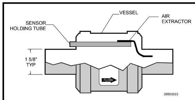
**Figure 11** - Checkit Refrigeration System Monitor
