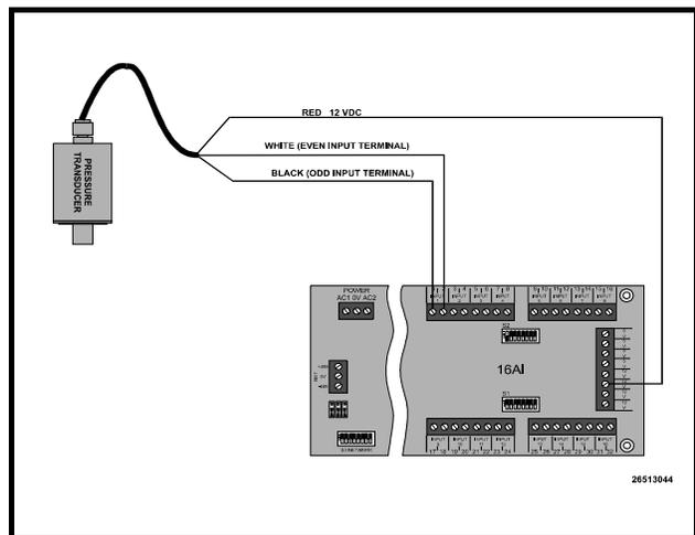
*Figure 27-Standard Pressure Transducer Wiring Diagram*
