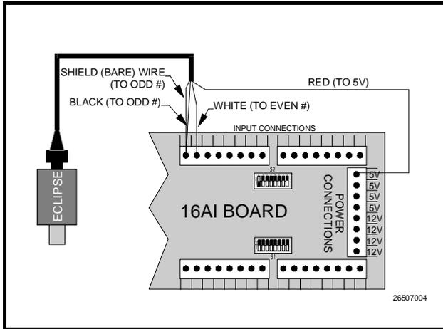
**Figure 26-**Typical Wiring Scheme for the Eclipse<sup>®</sup> Pressure Transducer
