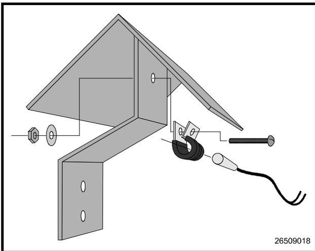
Figure 29-Outside Temperature Sensor with Cover and Clamp
