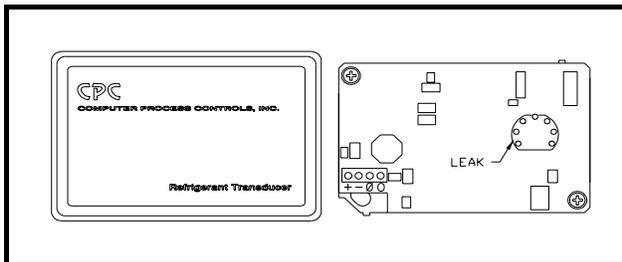
**Figure 23** - Refrigerant Transducer (Sensor Removed)
