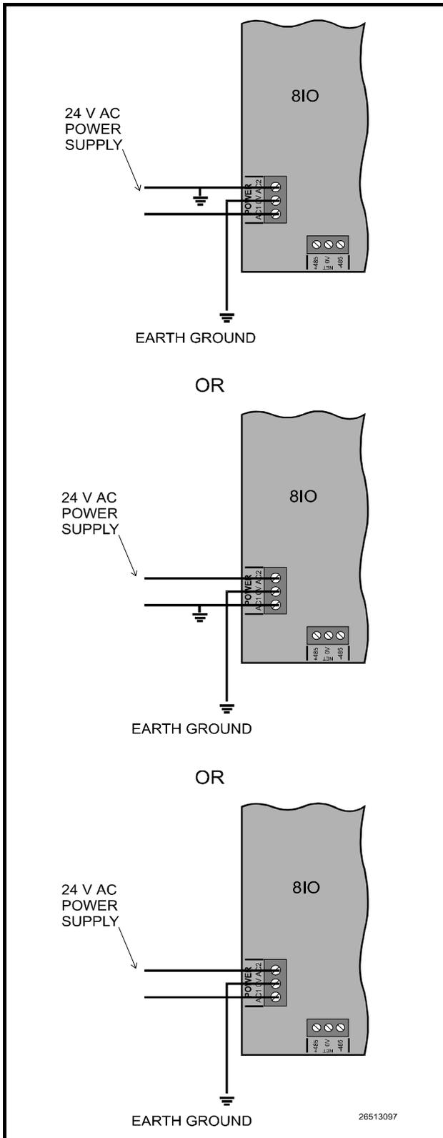
*Figure 41-One 8IO with a Ground on Either Side of the Power Supply and One 8IO with no Ground in the System*
