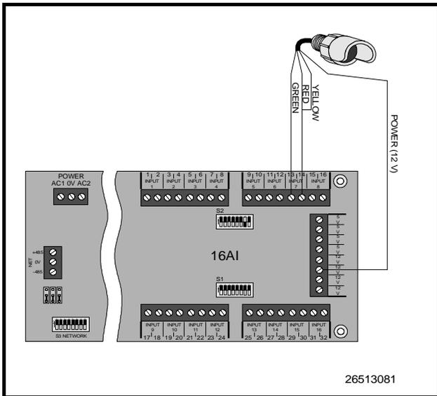
Figure 18-Light Level Sensor Wiring Diagram
