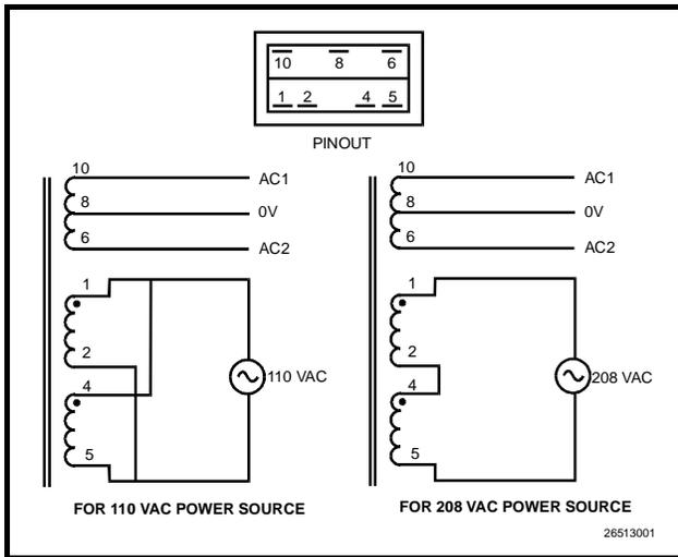
Figure 36 - Wiring for 640-0043, Three Board, and 640-0045, Six Board Transformer
