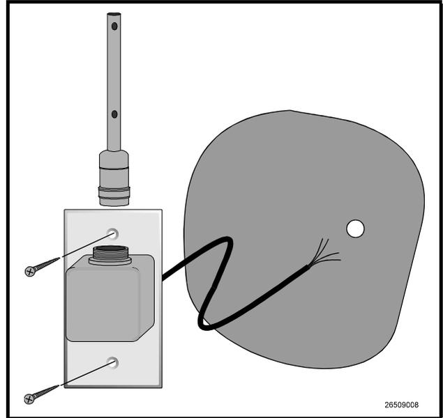
*Figure 15 -Dew Cell Dew Point Probe Mounting*
