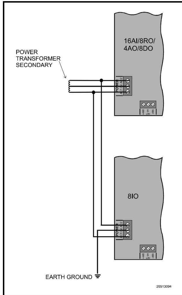
*Figure 40-8IO Board Wired in Combination with A or Multiple 16AI, 8RO, 4AO, 8DO*
