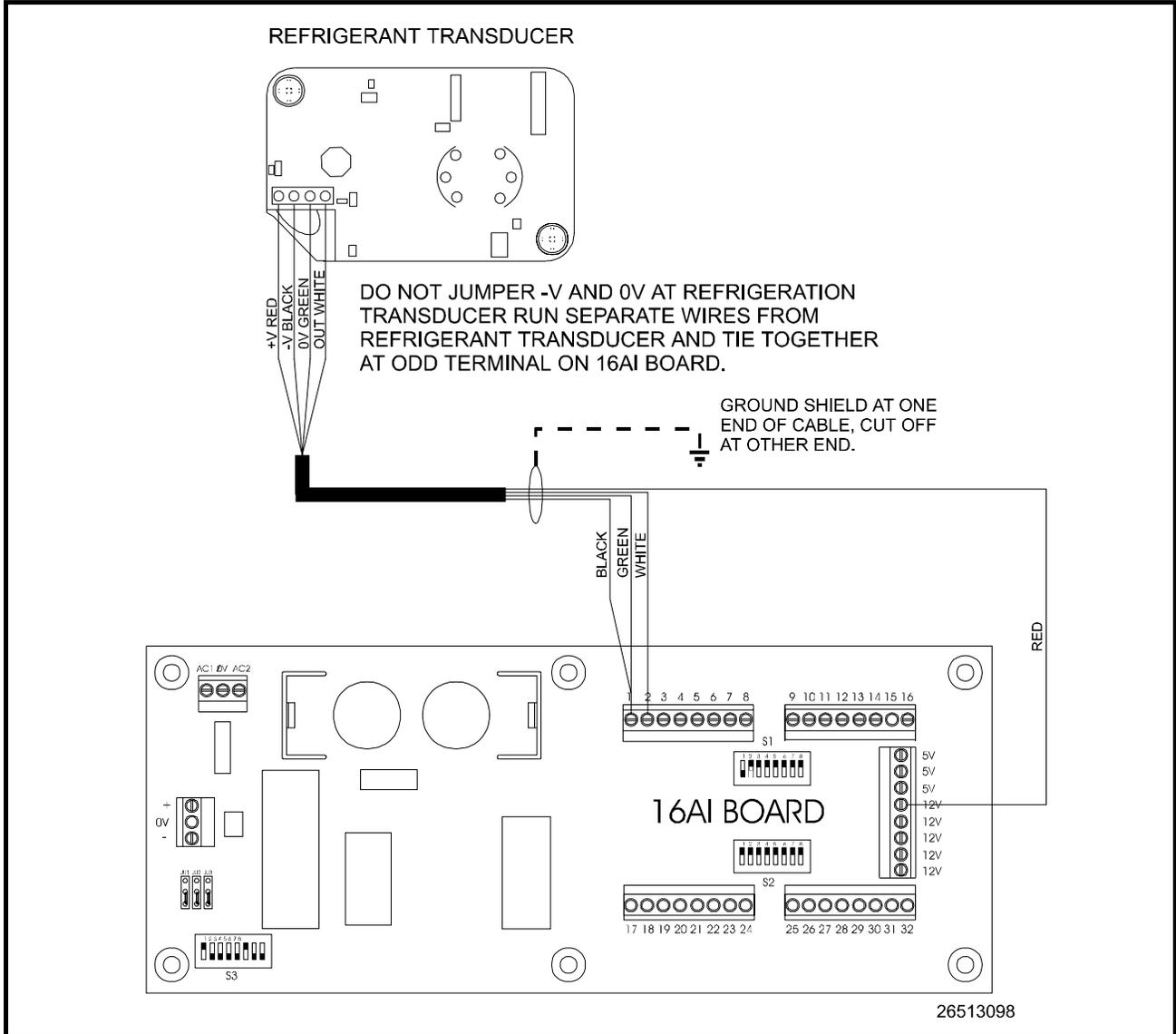
*Figure 24 - Single Refrigerant Transducer Layout*
