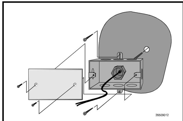
Figure 31-12-Inch Insertion Probe Mounting
