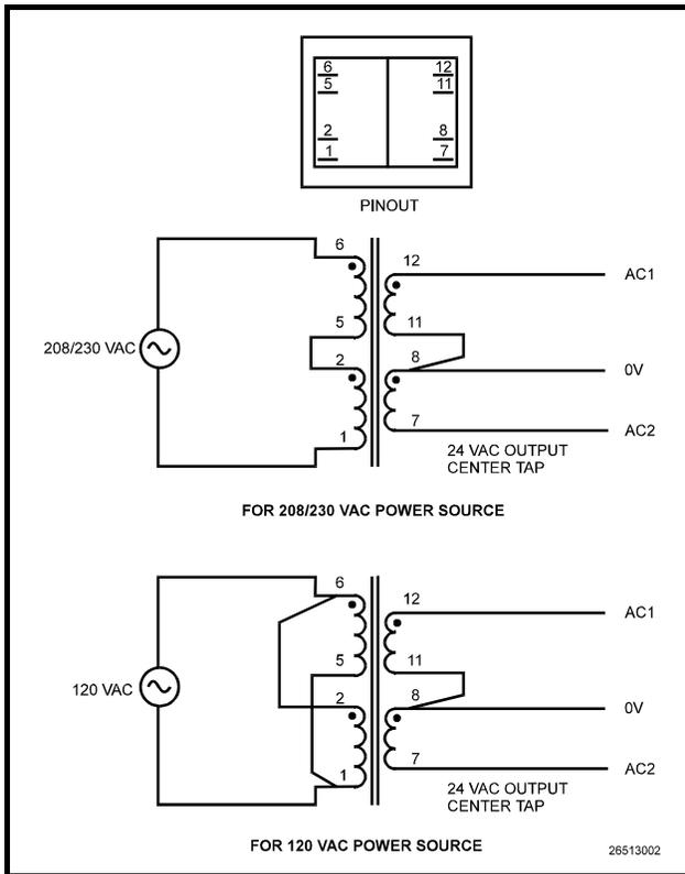
Figure 37 - Wiring for 640-0048, Ten Board Transformer
