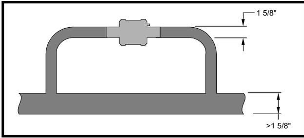
**Figure 13 - Installation of Checkit and Bypass for Lines Larger than 1 5/8"**
