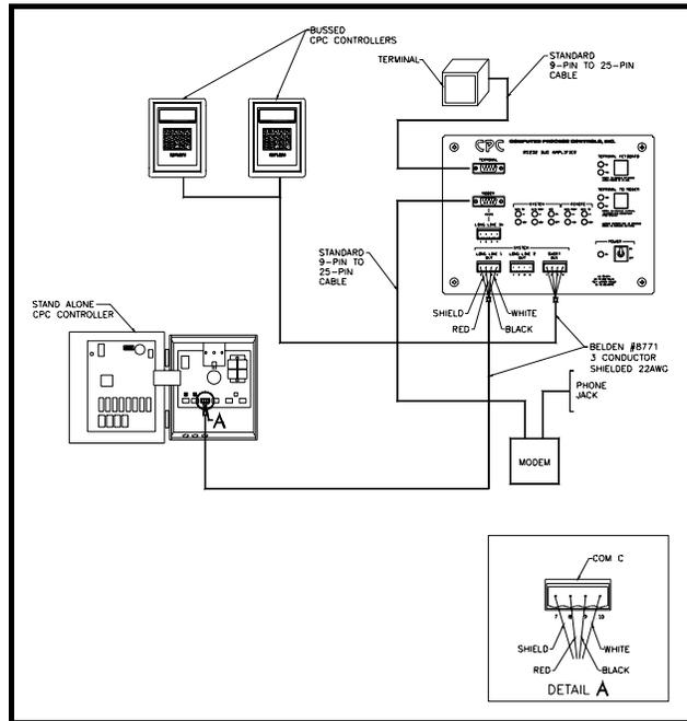
**Figure 6** - Typical Single-Amplifier Layout
