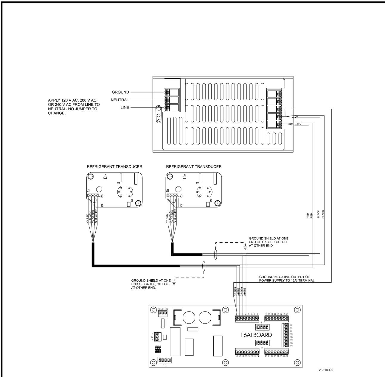
Figure 25 - Multiple Refrigerant Transducer Layout
