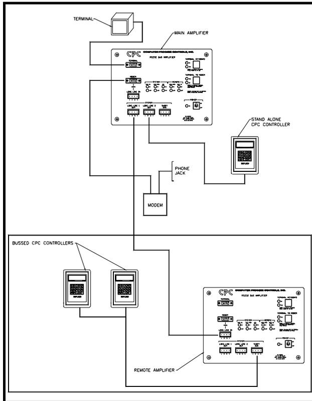
*Figure 7 - Typical Two-Amplifier Layout*
