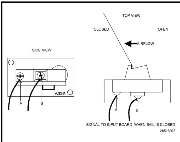
**Figure 42-S437A Switch Connection for Signaling When Airflow is Present**
