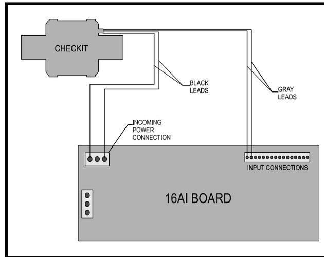
**Figure 14 - Checkit Typical Power Connections**
