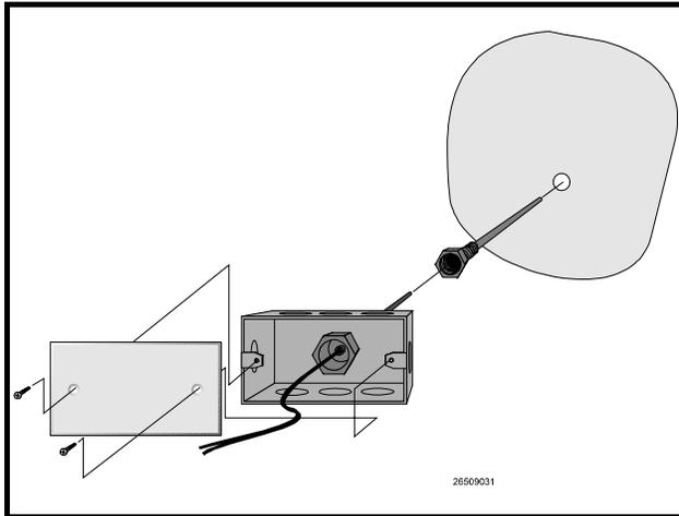
**Figure 32**-Immersion Probe with Sheath
