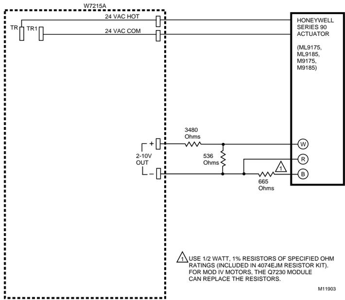
Fig. 1. W7215A used with Honeywell Series 90 Actuator.
