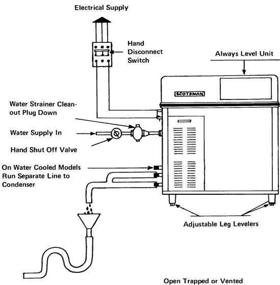
Open Trapped or Vented Drain. Recommend 1/4 Fall per foot of run on drain lines.
