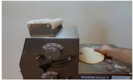
The rounded piece of dough comes out on the discharge tray.
