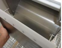
The #2 scraper lays on top of the bottom roll and is attached to the discharge tray as one piece.
