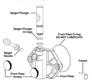
Fig. 3 Front Plate Assembly
